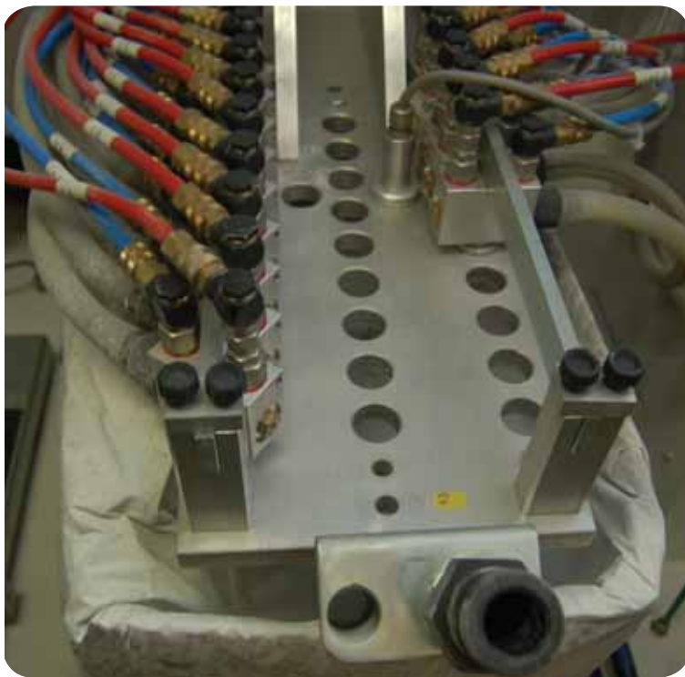
Powder is supplied to the guns by an automated feed center that pumps the powder directly from the box.
