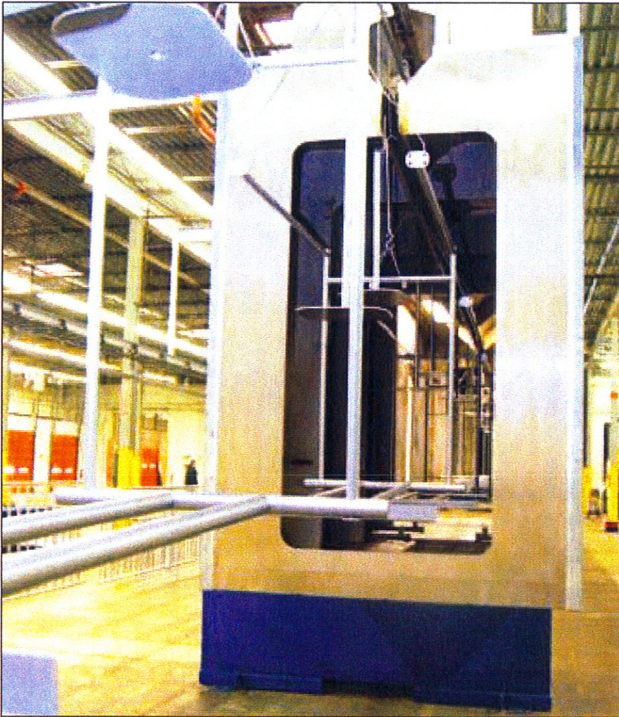
Parts enter the three-stage pretreatment system at Meyer Metals. Meyer left room to add additional stages for other processes in the future.
